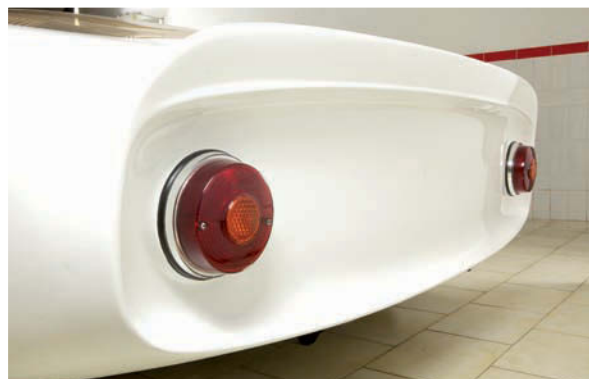
Short Kamm tail added to straightline speed and stability on fast US circuits. All-important chassis number proves this is one of four special 906Es
