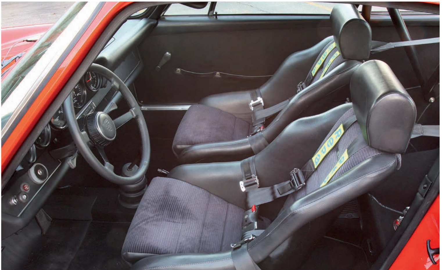
Seats are genuine ST items, as is the roll cage, the latter being supplied by Edmond Harris in the UK. Harnesses are Repa repros by Bill Rich Designs
